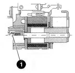
Checking multi-plate clutch
